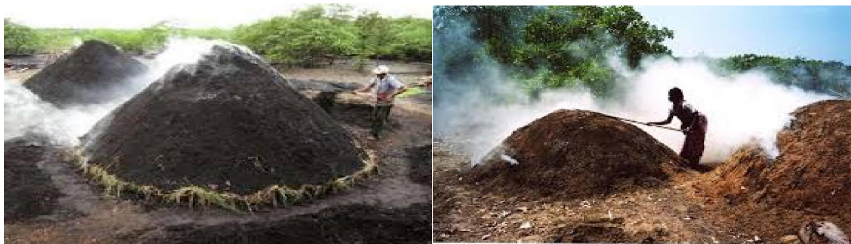
Figure 1: Earth Mound Method of Charcoal Production in Nigeria
