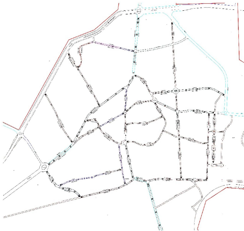
Figure 5. Dividing pavement sections to sample units
