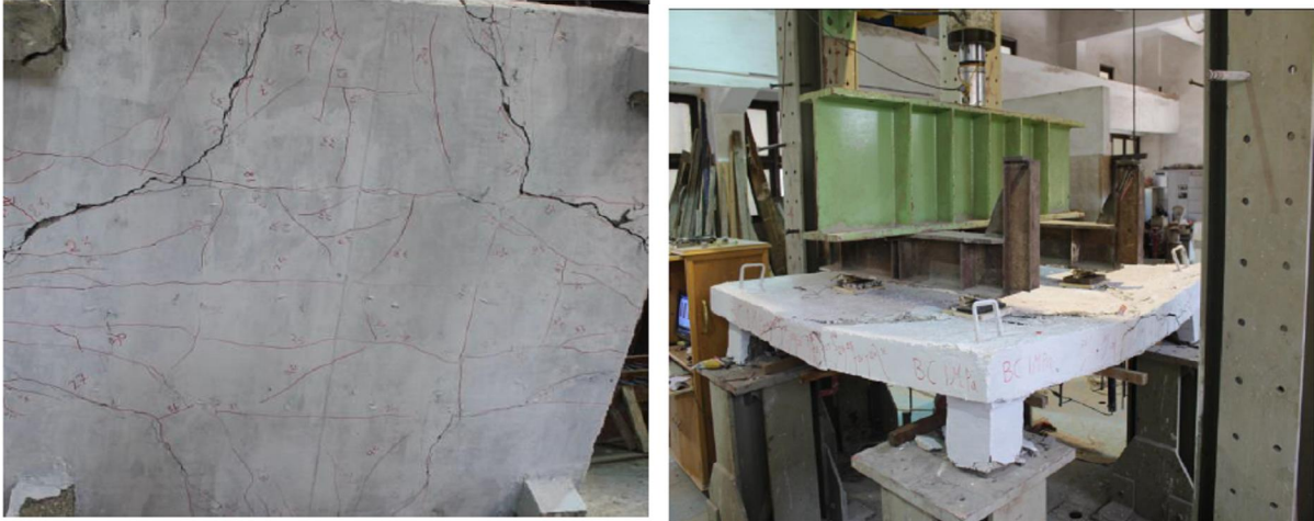
Fig. (8): Pattern of Crack, Concrete Crushing For BN
