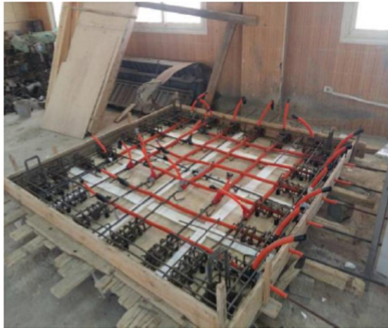
(a) Bonded Tendon Slab (1mpa) (b) Tendon Layout and Distribution
