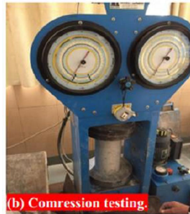
Fig. (5): Casting and testing standard cylinder of concrete.
