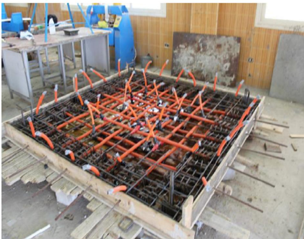
(a) Bonded Tendon Slab (2mpa) (b) Tendon Layout and Distribution.
