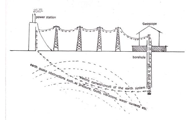
This is also easy study to recognize the impending earth quake. A borehole having suitable width and depth has to be dug. An earth wire or rod should be inserted into the underground by the borehole and linked with the concerned analysis section having apparatus to detect, compare measure of the electric currents of the electric circuit of the earth system. Otherwise by observing the home electric fans etc. we can study the electrogeopulsegram studies to predict the impending earth quake.
