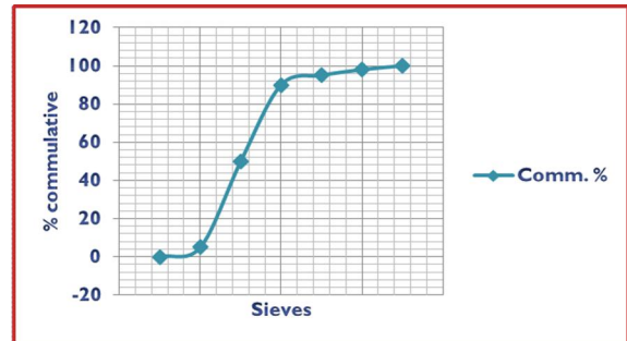
Figure 3: Gradation of the Cold Recycled Mixes
