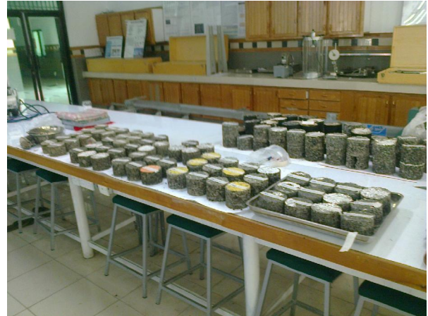
Figure 6. Laboratory Marshall Samples
