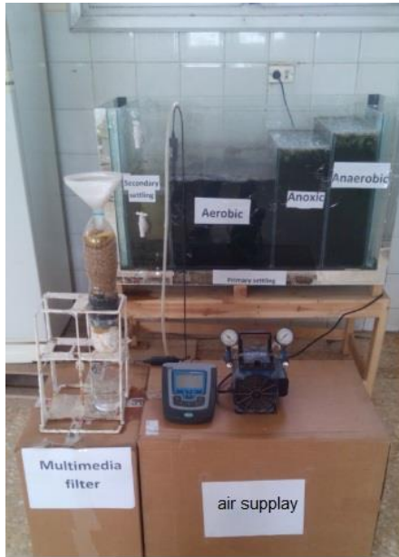
Fig (2) picture of the experimental pilot plant. Modified moving bed biofilm reactor, containing carriers in the anaerobic, anoxic and aerobic zones of the bioreactor (MBBR ).
