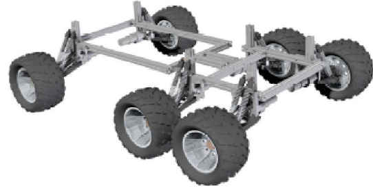
Figure 4: Chassis Frame, Monster Truck Suspension and Tires
