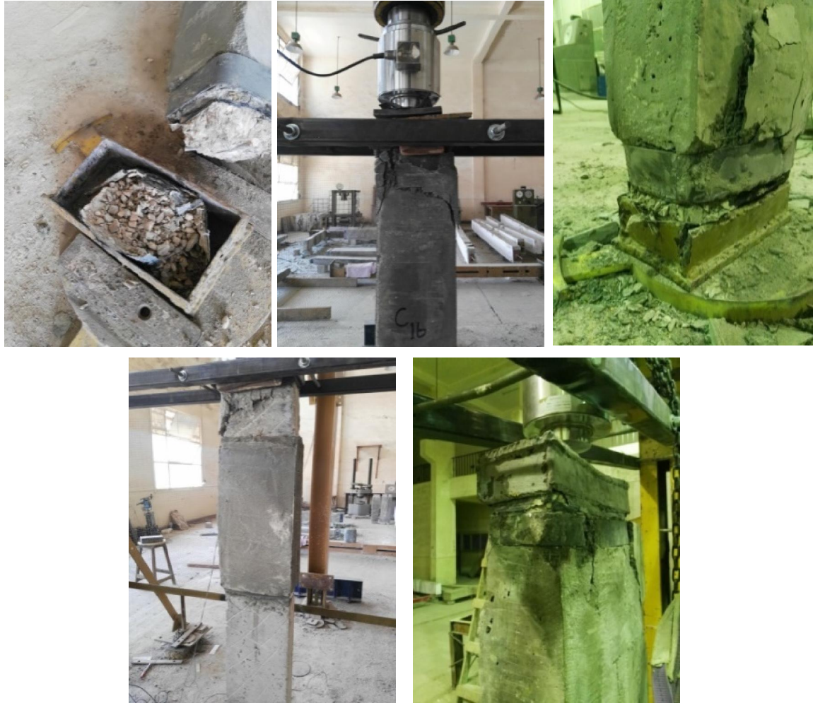
Figure [24] Damaged modes of retrofitted columns of the group (1) that retrofitted by [spiral stirrups \phi 6 /80mm+ three plies SWM]
