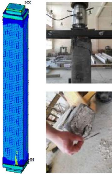
Figure [34] Comparison between modes of failure obtained from (FEA) and (EXP) for retrofitted column [C-1b] of group [1]
