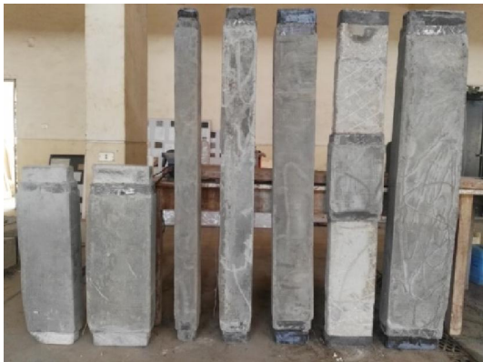
Figure [8] Retrofitted of both long and short column specimens before testing
