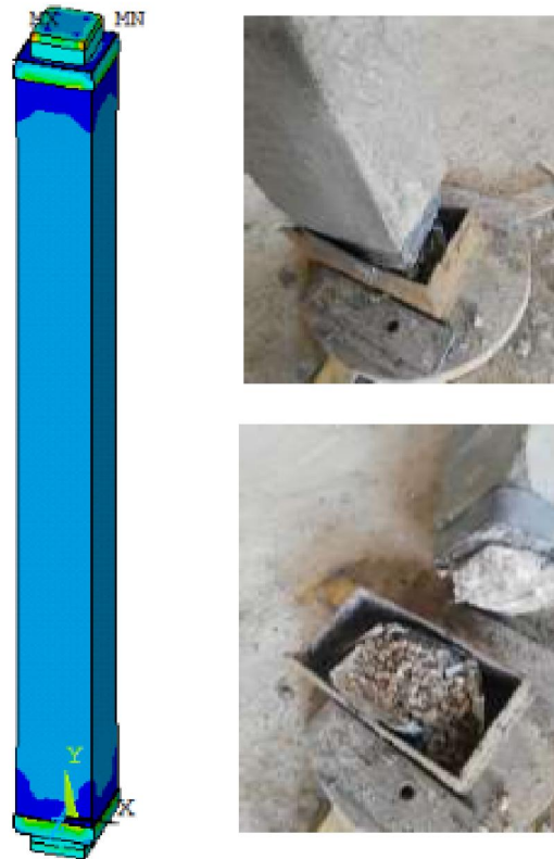
Figure [33] Comparison between modes of failure obtained from (FEA) and (EXP) for retrofitted column [C-1a] of group [1]
