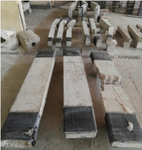
Figure [4] Specimens after testing before retrofitting
