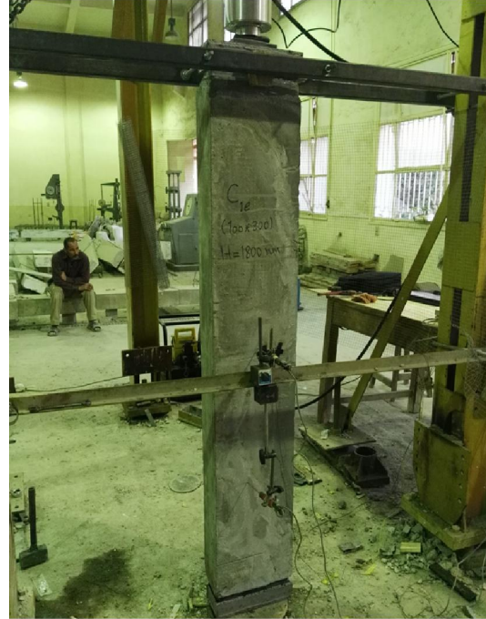
Figure [9] Loading frame and test set up
