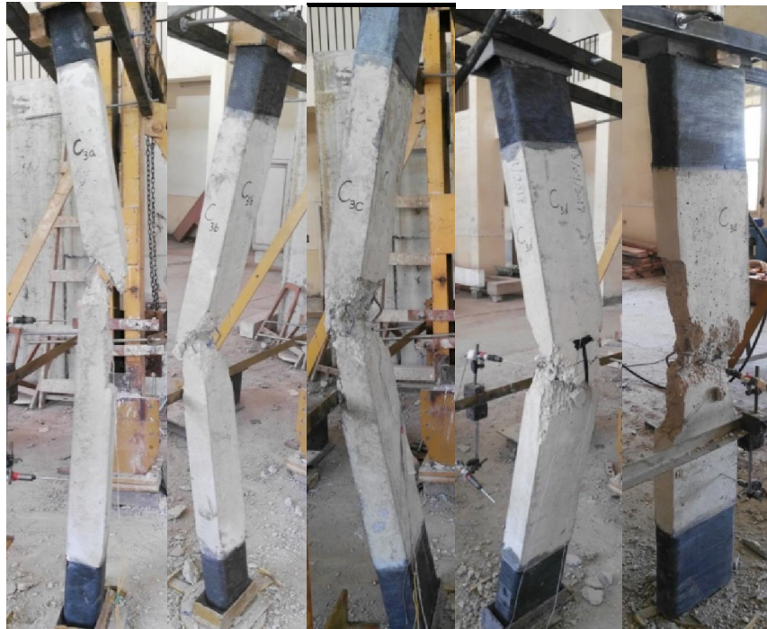
Figure [23] Damaged modes for tested control columns before retrofitting
