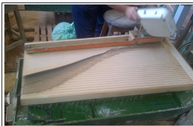
Fig. 3: The laboratory Wilfley shaking table (No.13)
