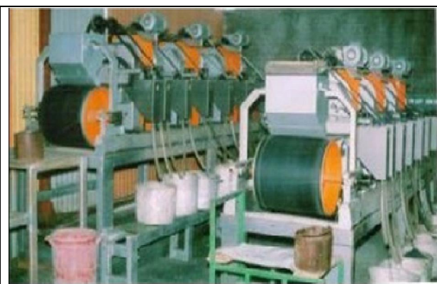
Fig. 4: Photograph of cross belt magnetic separator.
