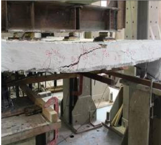
(a) Un Bonded Slab with CFRP Strip (USS) Concrete Crushing
