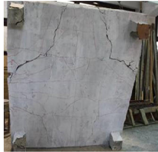
(a) Experimental Crack Pattern
