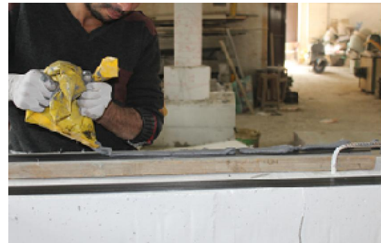
Fig. (10): Applied ADH4000 on CFRP strips
