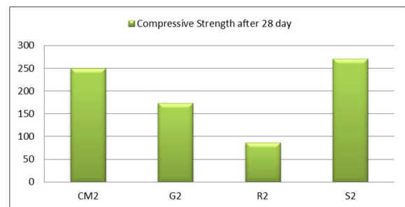
Figure 3. Compressive Strength of Concrete Mixes Containing 350 kg of Cement
