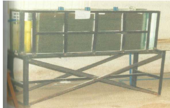
Figure 1a: 3-D Sand Tank Model. (Ojuri 2010)
