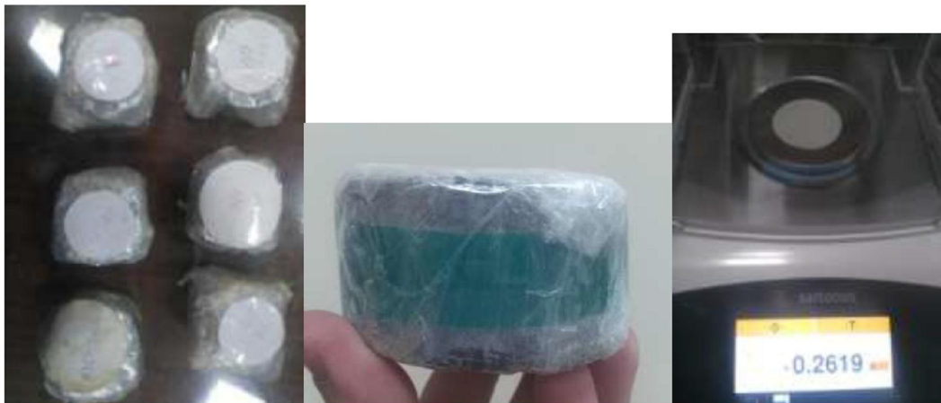
Fig.2 Suction Test Steps
