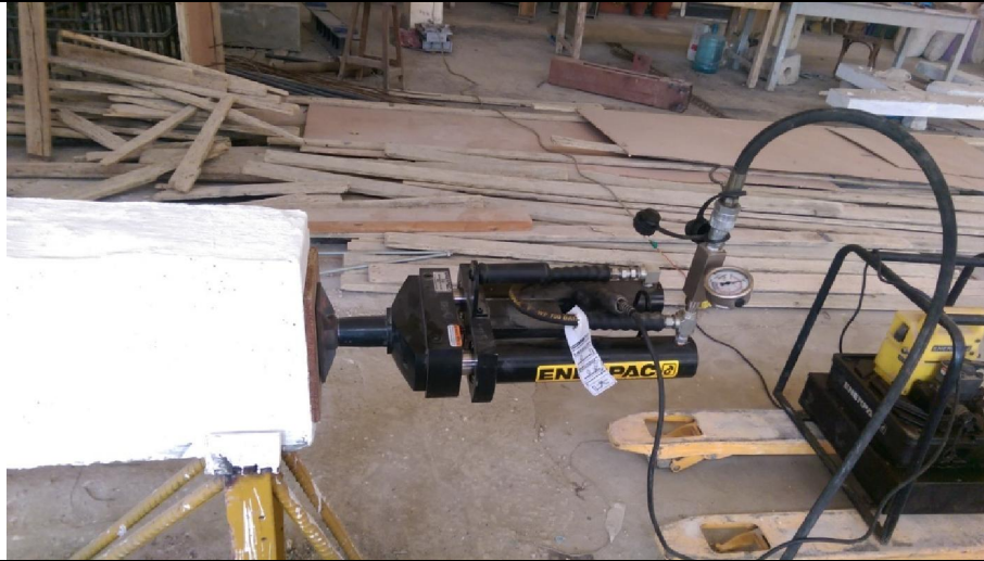
Fig (5) Pre-stressing process.
