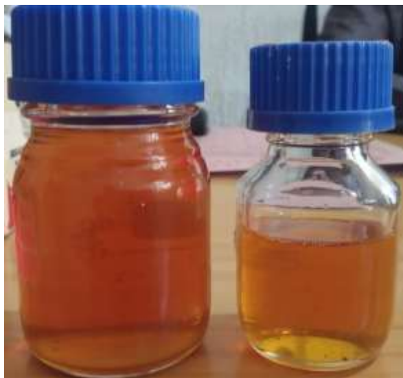
Figure 2. Oil-in-water nanoemulsion formulation of B. aegyptiaca seed kernel extract at 20:20:60 surfactant, oil, and water (SOW) ratio.
