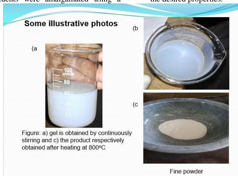
Figure 1: Barium Titanate gel and fine powder
