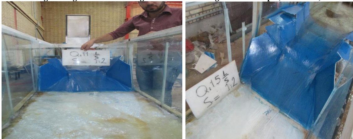
Fig 3. Built Long throat flume with 20 cm sill height and 1:2 slope (experimental)
