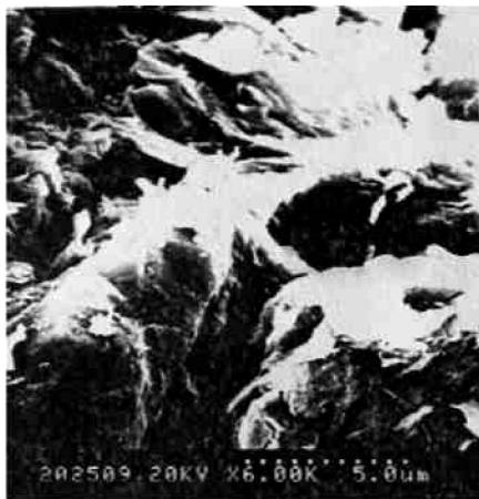
Fig. 1. Microstructure of loam (vd I-Sh) well 7, Chapt.4.65-4.95 after leaching at P = 0.4 \text{ MPa} .
