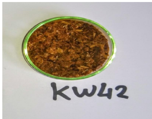
Figure 1. The dead biomass of Kw42 that was used for biosorption of \text{Cu}^{2+} , \text{Pb}^{2+} and \text{Cd}^{2+} from wastewater.
