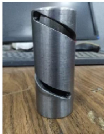
Figure 6 (a): Engraved cam sleeve (from different directions) Figure 6 (b) Sleeve dimensions Fig. 6 Parallel cam
