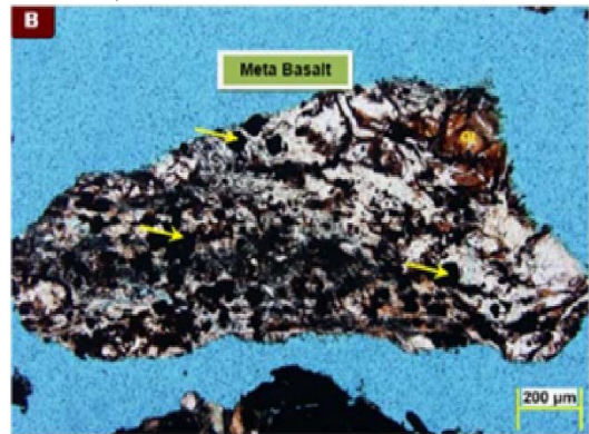
Figure 7: Ditch sample thin section at depth 13900 ft Upper Safa, SYRAH – 6Xst
