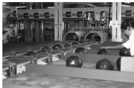
Figure 4. A devised system based on capacitive property for qualifying of watermelon (Kato, 1997).
