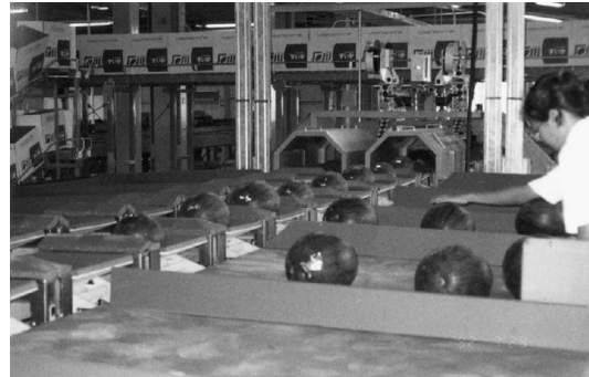
Figure 4. A devised system based on capacitive property for qualifying of watermelon (Kato, 1997).
