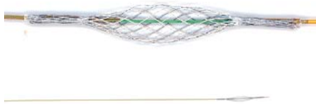
Figure 1. (Top) Basket catheter tip with expanding mesh that brings the thermistors in contact with the arterial wall. (Bottom) full catheter body (4F) that can be advanced from the femoral vein to map the temperature of the entire aorta.
