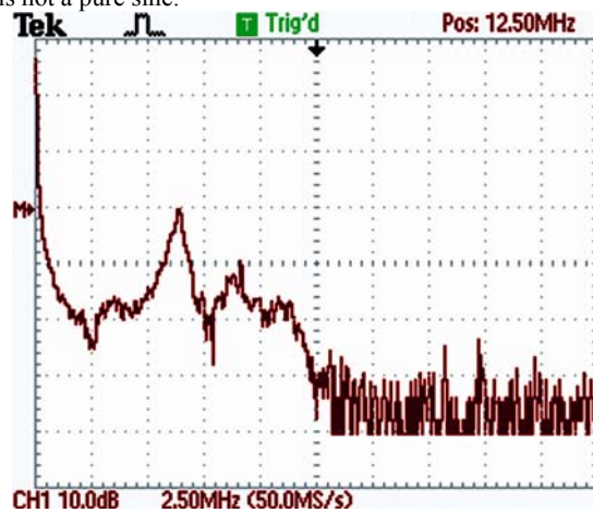
Figure 8 The frequency spectrum of the pulsed MF induced, with bandwidth reaching 12.5MHz.
