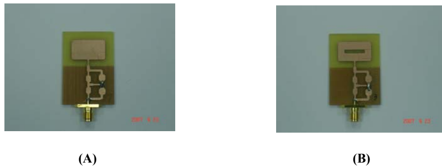
Figure 3. Prototype of the proposed antennas in design (A) with slot (B) without slot
