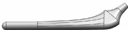
Figure 9. Solid model of a femoral stem built by Unigraphics NX. (Type I)
