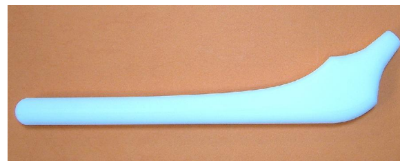
Figure 13. Rapid prototyped model of a femoral stem produced through FDM process. (Type I)
