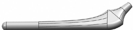
Figure 9. Solid model of a femoral stem built by Unigraphics NX. (Type I)
