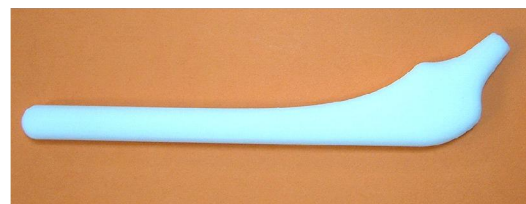
Figure 14. Rapid prototyped model of a femoral stem produced through FDM process. (Type II)
