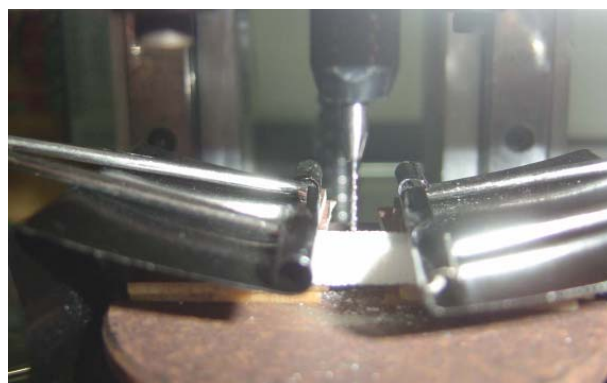
Fig. 2. Experiment setup in a micro drill with bones
