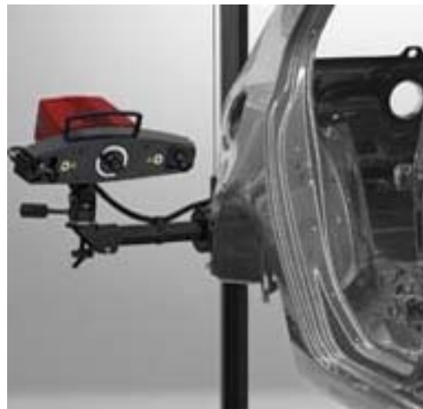
Figure 1. ATOS non-contact laser scanning system
