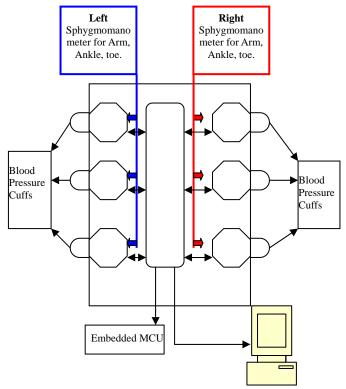
Figure 4. Synchronous TBI and ABI measurement scheme
