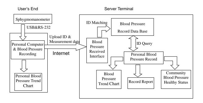
Figure 6. The Sphygmomanometer measurement and transmission block diagram
