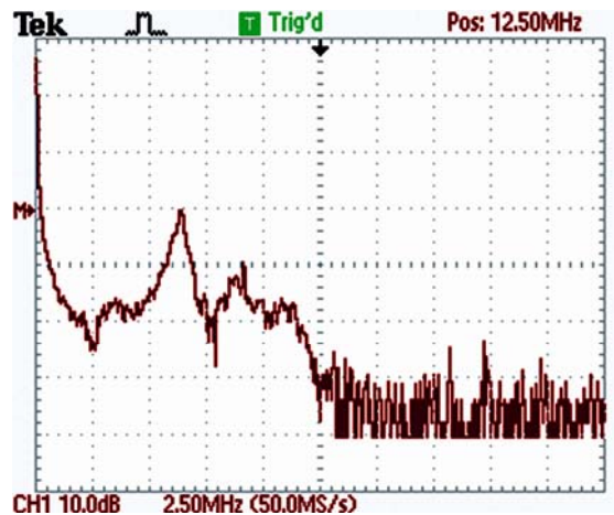
Figure 8 The frequency spectrum of the pulsed MF induced, with bandwidth reaching 12.5MHz.
