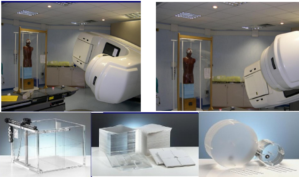
Figure (1): The setup for Humanoid Phatom in upper and lower position for gantry rotation respectively and phantom for measurement.
