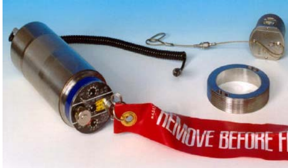
Fig. 3. A sample missile fuze adopted from Cope [10].
