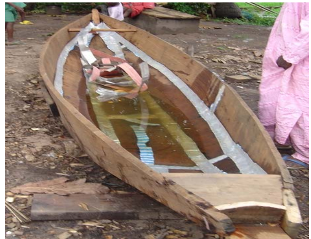
Plate 2.4: A newly constructed planked canoe with strips of galvanized iron/aluminum
