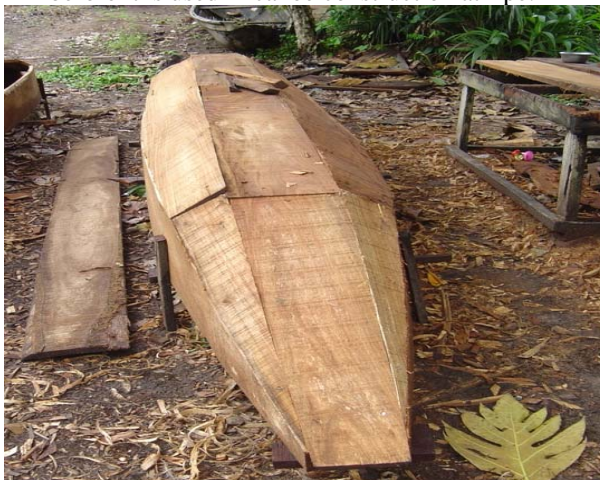
Plate 2.3: New constructed planked canoe at Epe (back hull)
