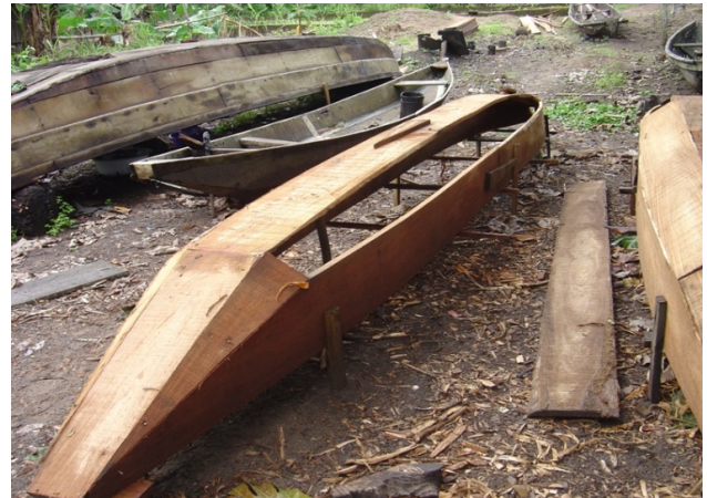
Plate 2.2: Planked canoe under construction at Epe.
