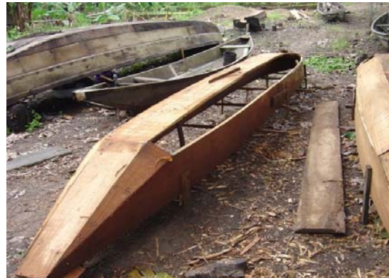
Plate 1.2: Planked canoe under construction at Epe.
