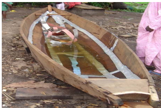
Plate 1.4: A newly constructed planked canoe with strips of galvanized iron aluminum
