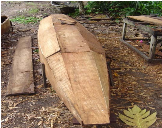
Plate 1.3: New constructed planked canoe at Epe (back hull)
