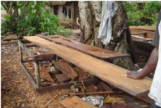
Plate 1.1: Planks placed on attender for framing before it is used in canoe construction at Epe.
