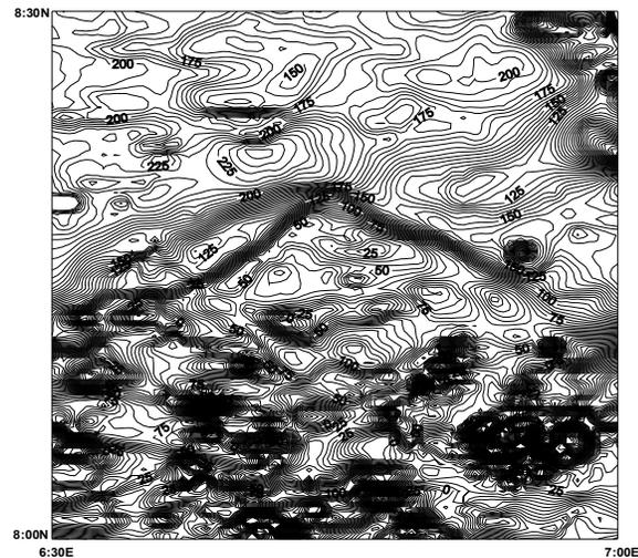
**FIG: 2b** Total field aeromagnetic anomaly map of koton- karifi area(sheet 227). The main field in form of igrf (igrf model 1975 of epoch date 1 january 1974) has been removed. Contour interval is 5nT.
