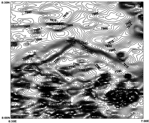
**FIG: 2a** Total Field Aeromagnetic Map (Sheet 227) of Koton Karifi. Contour interval is 5 nT. Actual values are obtained by adding 25000 nT to contour values. Regional correction based on IGRF (epoch date 1st January 1974) has not been made.
