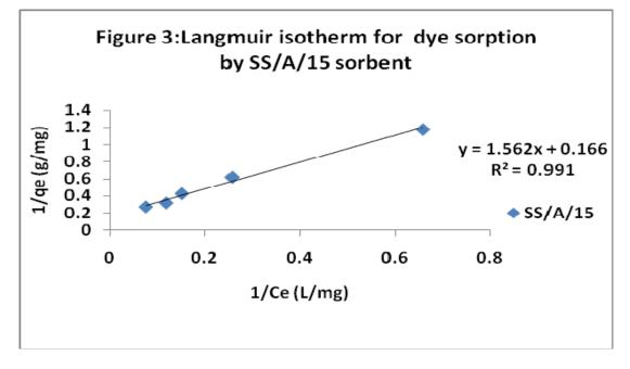
The Langmuir constant, relating to the maximum adsorption capacity  $(q_m)$  was investigated. Sorbent, SS/A/15 gave the highest value for maximum adsorption capacity (6.124 mgg<sup>-1</sup>). This is in agreement with the highest adsorption capacity value present by acidic sorbents from the Freundlich constants ( $k_f = 0.646$ ). This work uncovered the fact that the maximum adsorption capacity of any series
