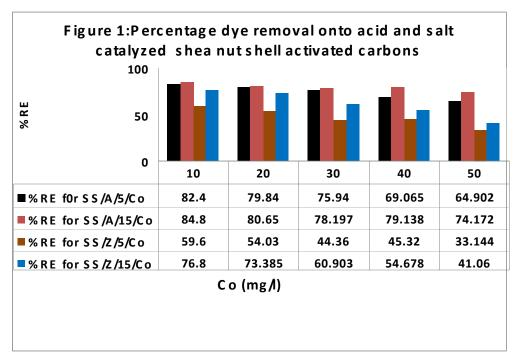
The % dye removal by the four sorbent series follows the order, SS/A/15 > SS/A/5 > SS/Z/15 > SS/Z/15. Results in this study revealed that biomass activated at a longer dwell time (15 minutes) gave higher percents dye uptake (74.172-84.800 %). ZnCl<sub>2</sub> is a less favorable activating agent especially when cracking or pyrolysis is done at short dwell time. This
