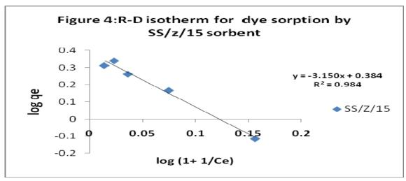
Just like the Freundlich adsorption capacities  $(k_f)$ , it was revealed that the theoretical adsorption capacity  $(q_D)$  from the R-D isotherm were also lower in magnitude than the Langmuir maximum adsorption
