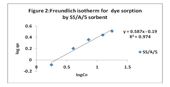
The degree of heterogeneity of adsorption surface was also measured from the 1/n values. According to Hameed *et al.*, (2006) the Freundlich equation slope (1/n), ranging between 0 and 1 is a measure of
